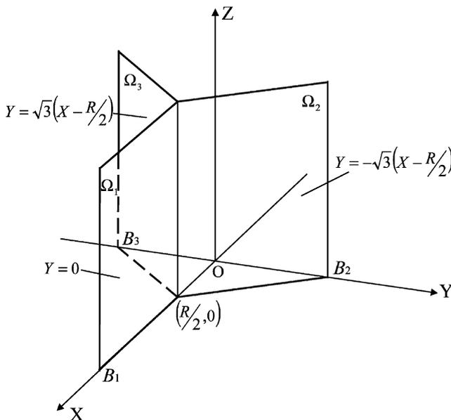
Fig. 3. Illustration of the three constraint planes.
