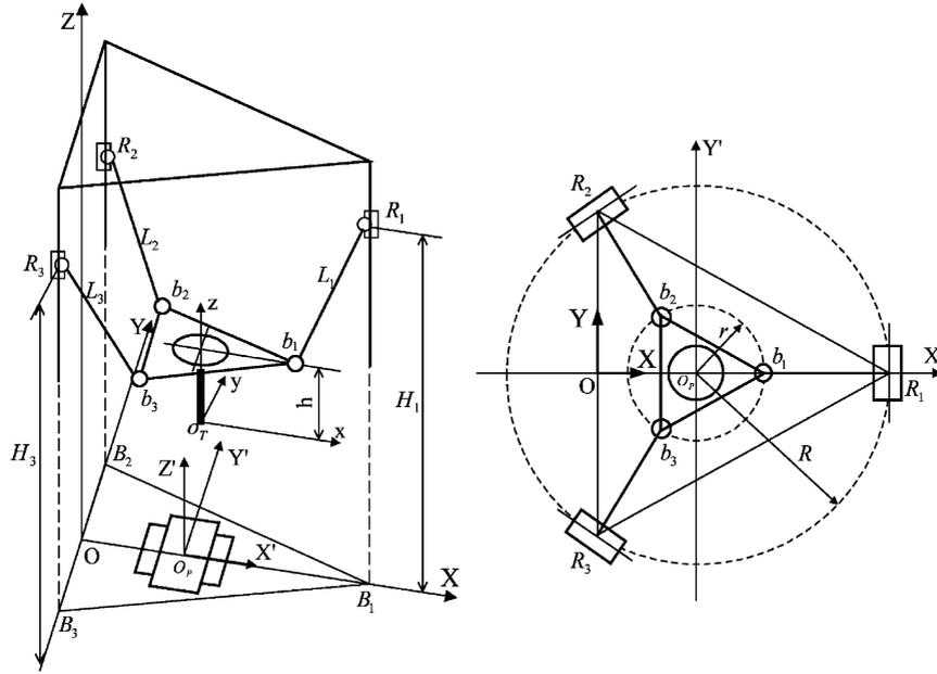
Fig. 2. Schematic diagram of the serial-parallel structure.
