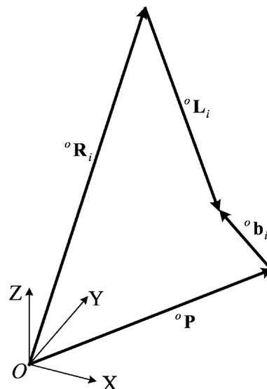
Fig. 4. Close loop of linkage  $i$  of the machine tool structure.
